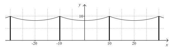
The cable between the middle two poles can be modelled by  $y = e^{x/8} + e^{-x/8} + a$  where  $a \in \mathbb{R}$ .
