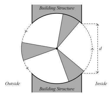
The angle subtended by each compartment is three times the angle subtended by each circular segment.
